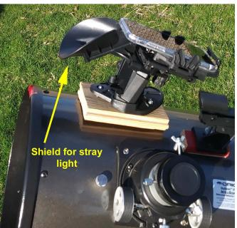
The bracket is shaped to fit a much smaller tube, so I fastened it to a wood block, which is secured to the tube with foamy 2-sided tape.
