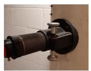
The tall rack and pinion focuser is for 2 inch eyepieces but comes with a 1 1/4 inch adapter. It is mounted to an adapter plate that matched to the curvature of the tube.
